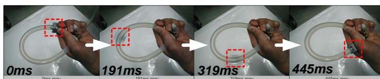
Photo.1 Movement of tested flexible pneumatic cylinder
