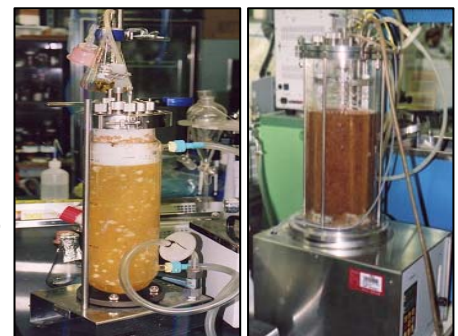
Fig.5 Production of gelatin-like compound in Air-lift type fermenter and Jarfermenter
